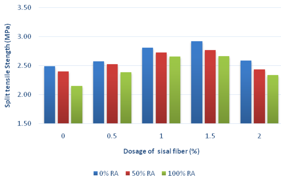
Figure 3: Variation split tensile strength with sisal fibers and recycled aggregate
