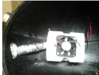
Fig:- fix the fan with cooling chamber
