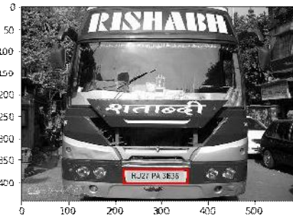
(c) Candidate rectangles after approximating from contours
