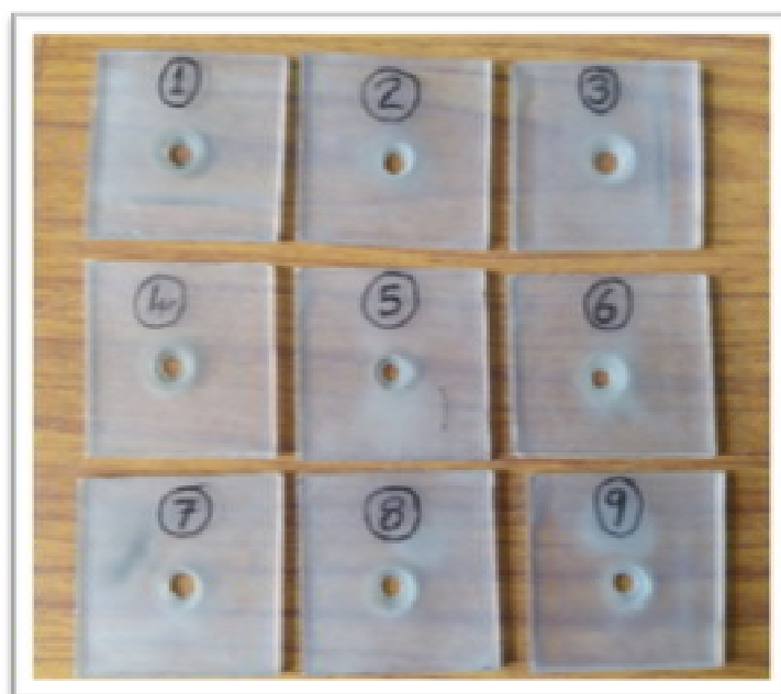
Figure : 10PMMA specimen after HAJM
