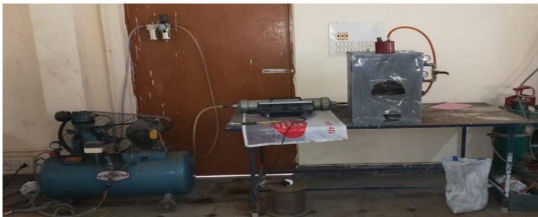
Figure 1: Hot air abrasive jet machine
