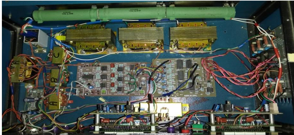
Fig. 8 The hardware testing circuit of six-pulse converter
