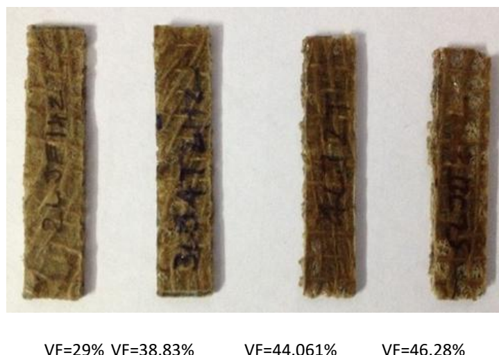
Figure 4. Fig. of samples used in the DMA test (all dimensions in mm).
