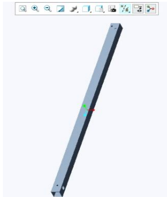
Fig 4.1 Creo model of base used in portable material handling machine
