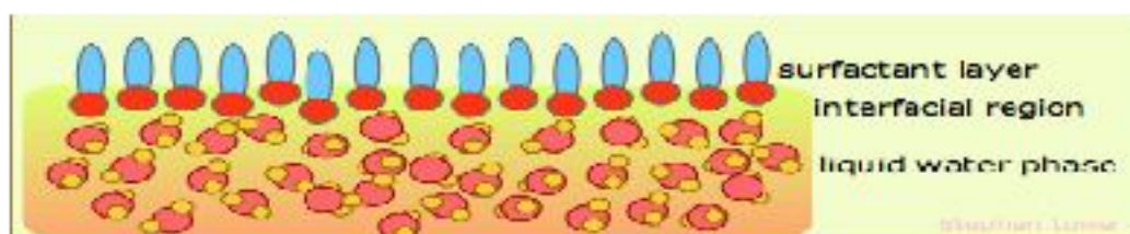
Fig1. How surfactant reduces surface tension of liquid
