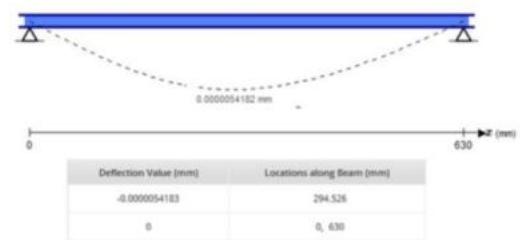
Fig-9- SFD, BMD, and deflection curves of base plate from SKYCIIV
