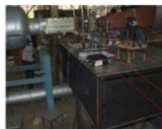
Fig-15-Arrangement of apparatus on traverse at combustion test rig
