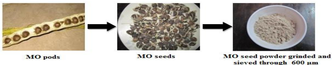
Fig.1. Preparation steps of Moringaoleifera seed powder
