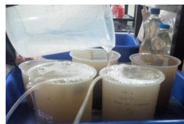
Fig. 1 B (1&2)- Showing aerator procedure for separation of particles from soil
