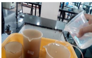
Fig. 1 B (1&2)- Showing aerator procedure for separation of particles from soil
