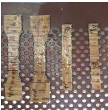
Fig.9 Tensile test & Flexural Test-Jute/Sisal.
