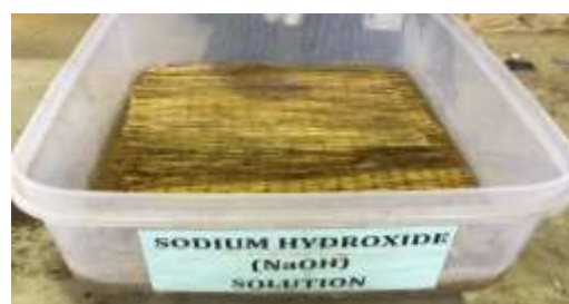
Fig.5. Fiber mat soaked in NaOH Solution
