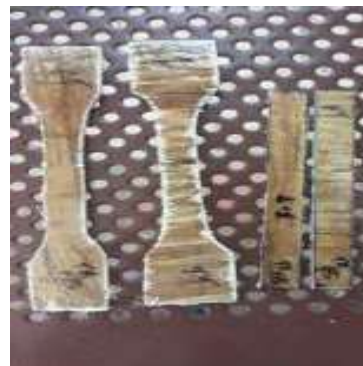
Fig.10 Tensile test & Flexural Test-Flax/Sisal.
