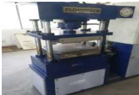
Fig 5 Compressing using Hot Press Moulding
