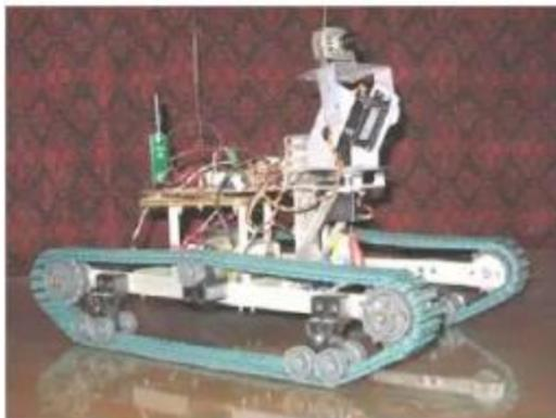
Fig. 5 The complete robot unit with the pan-and-tilt mechanism for better navigation
