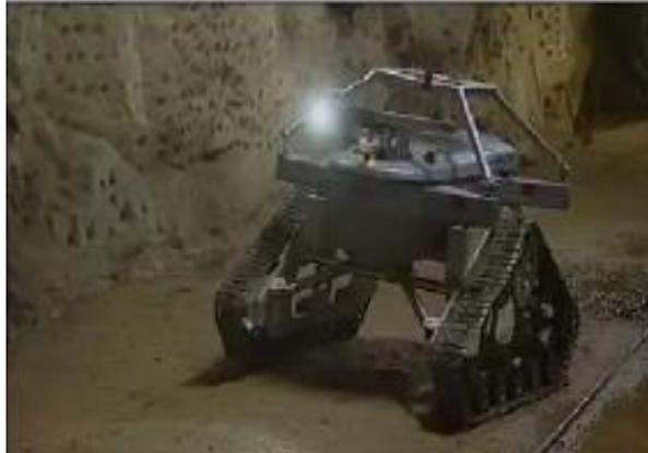
Fig.10. Robotic system for path finder in underground mines
